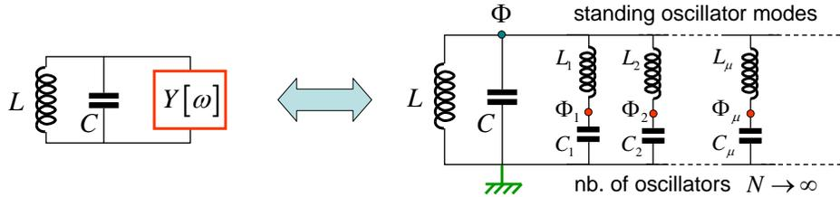
$$\hat{H} = \frac{\hat{\Phi}^2}{2L} + \frac{\hat{Q}^2}{2C} + \sum_{\mu=1}^N \left[ \frac{\hat{Q}_{\mu}^2}{2C_{\mu}} + \frac{(\hat{\Phi}_{\mu} - \hat{\Phi})^2}{2L_{\mu}} \right] \quad \text{Re}[Y[\omega_{\mu}]] = \sqrt{\frac{C_{\mu}}{L_{\mu}}} \quad \omega_{\mu} = \sqrt{\frac{1}{L_{\mu}C_{\mu}}}$$
