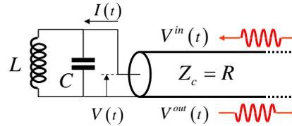
$$\begin{cases} V(t) = \dot{\Phi}(t) = R(I_D(t) + I_N(t) - I(t)) \\ C\ddot{\Phi} + \frac{\dot{\Phi}}{R} + \frac{\Phi}{L} = I_D(t) + I_N(t) \end{cases}$$
