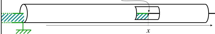
Lagrangian density:  $\mathcal{L}(x) = \frac{C_\ell}{2} \left( \frac{\partial \Phi}{\partial t} \right)^2 - \frac{1}{2L_\ell} \left( \frac{\partial \Phi}{\partial x} \right)^2$
