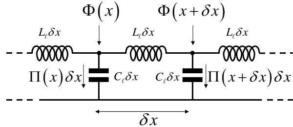
$$\left[ \Phi(x), \Pi(x)\delta x \right] = i\hbar \quad \left. \begin{array}{l} \\ \end{array} \right\} \xrightarrow{\delta x \rightarrow 0} \left[ \hat{\Phi}(x_1), \hat{\Pi}(x_2) \right] = i\hbar \delta(x_1 - x_2)$$
