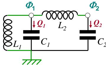
$$\hat{H}(\hat{\Phi}_1, \hat{Q}_1; \hat{\Phi}_2, \hat{Q}_2) = \frac{\hat{Q}_1^2}{2C_1} + \frac{\hat{\Phi}_1^2}{2L_1} + \frac{\hat{Q}_2^2}{2C_2} + \frac{(\hat{\Phi}_2 - \hat{\Phi}_1)^2}{2L_2}$$
