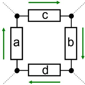
$$\sum_{\text{branches } \lambda \text{ around loop}} V_{\lambda} = 0$$
