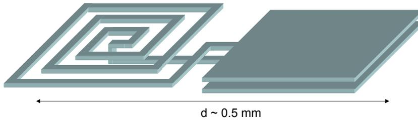
MICROFABRICATION →  $L \sim 3 \text{ nH}$ ,  $C \sim 1 \text{ pF}$ ,  $\omega_r / 2\pi \sim 5 \text{ GHz}$
