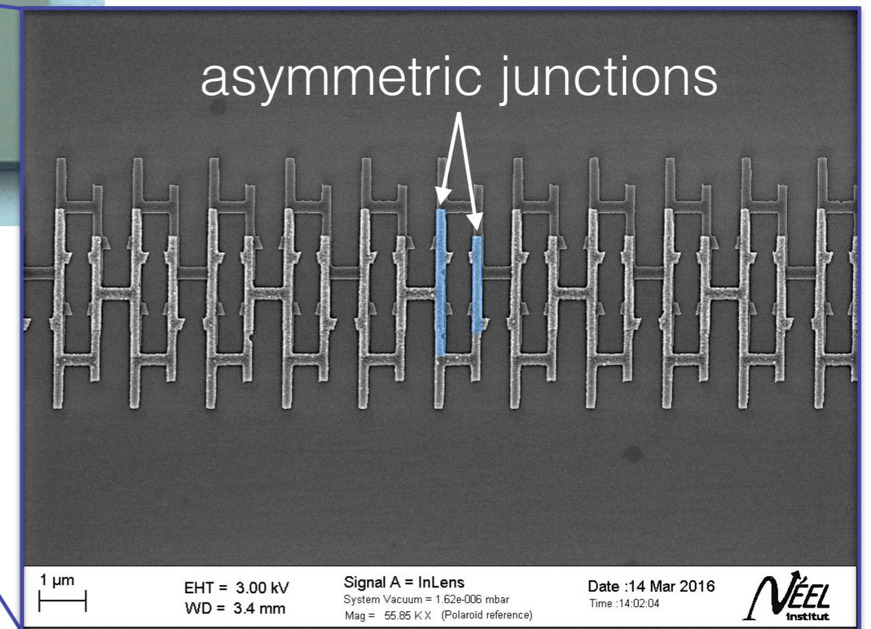
Challenges faced: stitching errors, resist homogeneity, focus homogeneity, proximity effect....
